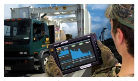
The spectroscopy detector is configured to collect gamma interactions in the energy range from 50 keV to 3 MeV. It provides statistically accurate dose rate
